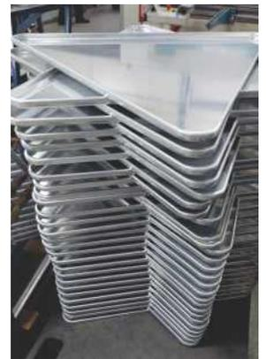
Bending edges is done around the whole sign base plate, without cease
