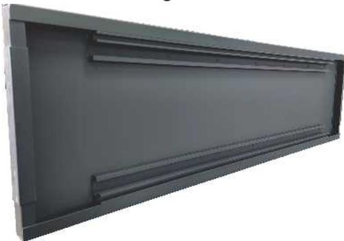
Rigidity of this type of large traffic signs is achieved by bending their edges and by installation of the aluminium profiles on their back. Large signboards are made of segments connected together on the pillars
