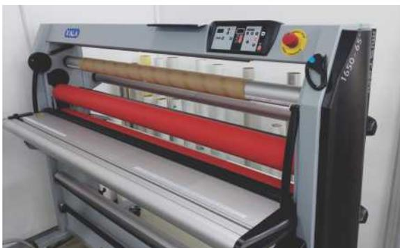
Printed material needs to be overlaminated with special laminating material to provide UV and other protection of printed application. For that, we use quality machine capable of providing what is needed based on demands from material producer.
