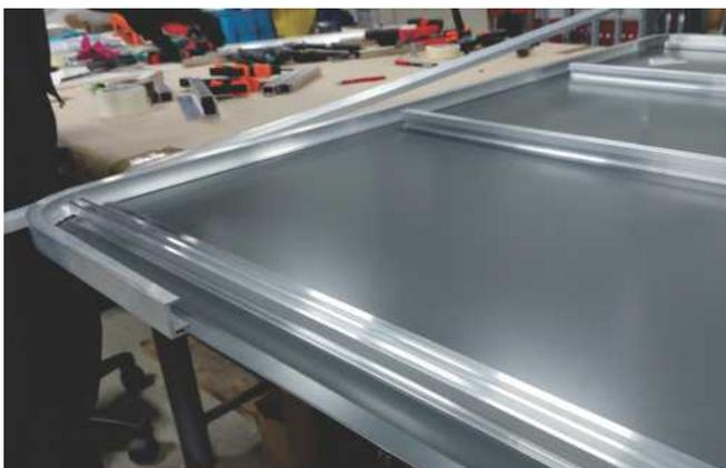
Aluminium frame 35mm wide reinforce aluminium signpost all around its edges.
